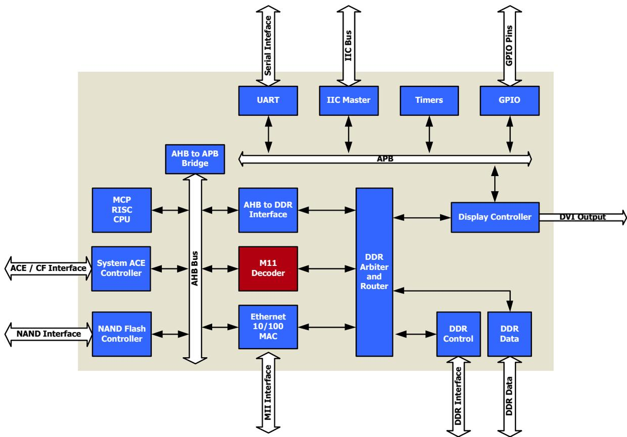
Using the integrated Compact Flash system, custom bit streams may be loaded into memory and decoded using either customer developed software or the included DV video player. The video output system makes use of the on-board DVI interface and requires no additional daughter cards.
