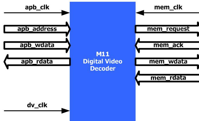
The M11 decoder core includes standard interfaces for host CPU access and frame store manipulation. Taking advantage of the modular nature of the design, Trilinear Technologies offers custom interfaces which conform to customer specifications. The modification of the interfaces requires no additional changes to the core decoding functions.
